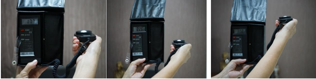
Figure 33 one light on 177 lux two light on 226 lux three light on 302 lux
