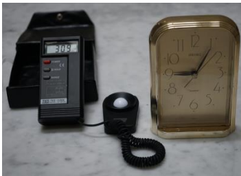
Figure 34: Non-Air conditioned Illumination 309 lux
