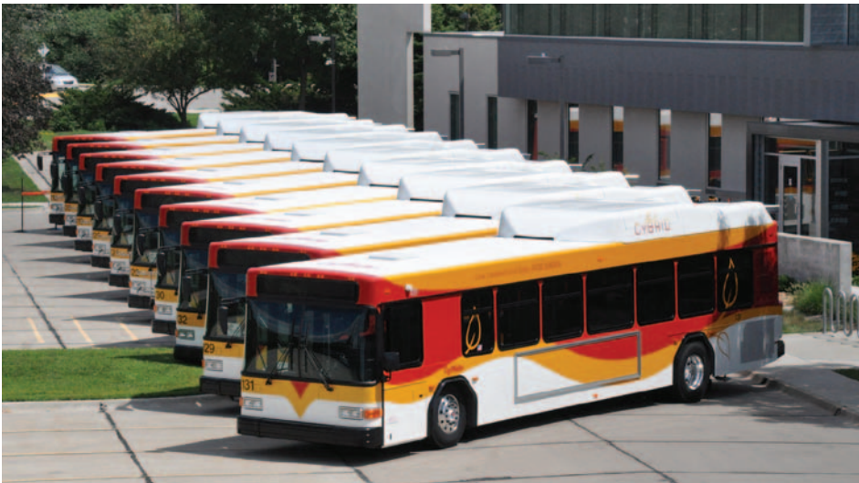
CyRide's ten new "CYBRID" buses use both hybrid technology and alternative fuel (biodiesel), a first for the transit agency.
